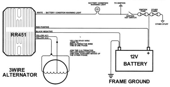
Problems with poor charging are usually caused by poor connections, or by not connecting **RED POSITIVE** & **BLACK NEGATIVE** wires DIRECTLY to the battery.
